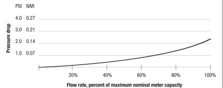
h Based on metering safety solvent, approximate viscosity 30 SSU (1 centipoise). When meter is operated at 100% capacity, the average pressure drop on safety solvent at 30 SSU (1 centipoise) will be approximately 2.3 PSI. When operated at 50% capacity, average pressure drop will be approximately 0.6 PSI (0.04 BAR).
